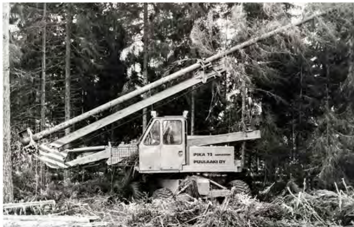
◆ Timber harvesting became rapidly mechanised in the 1970s. Chainsaws were accompanied by processors, which trimmed and cut stems felled by loggers. Gradually machines were developed that could cut standing stems as well. Puulaki Oy's Pika 75 in operation. Lasse Säteri, the Metsäteho Collection, Lusto.
