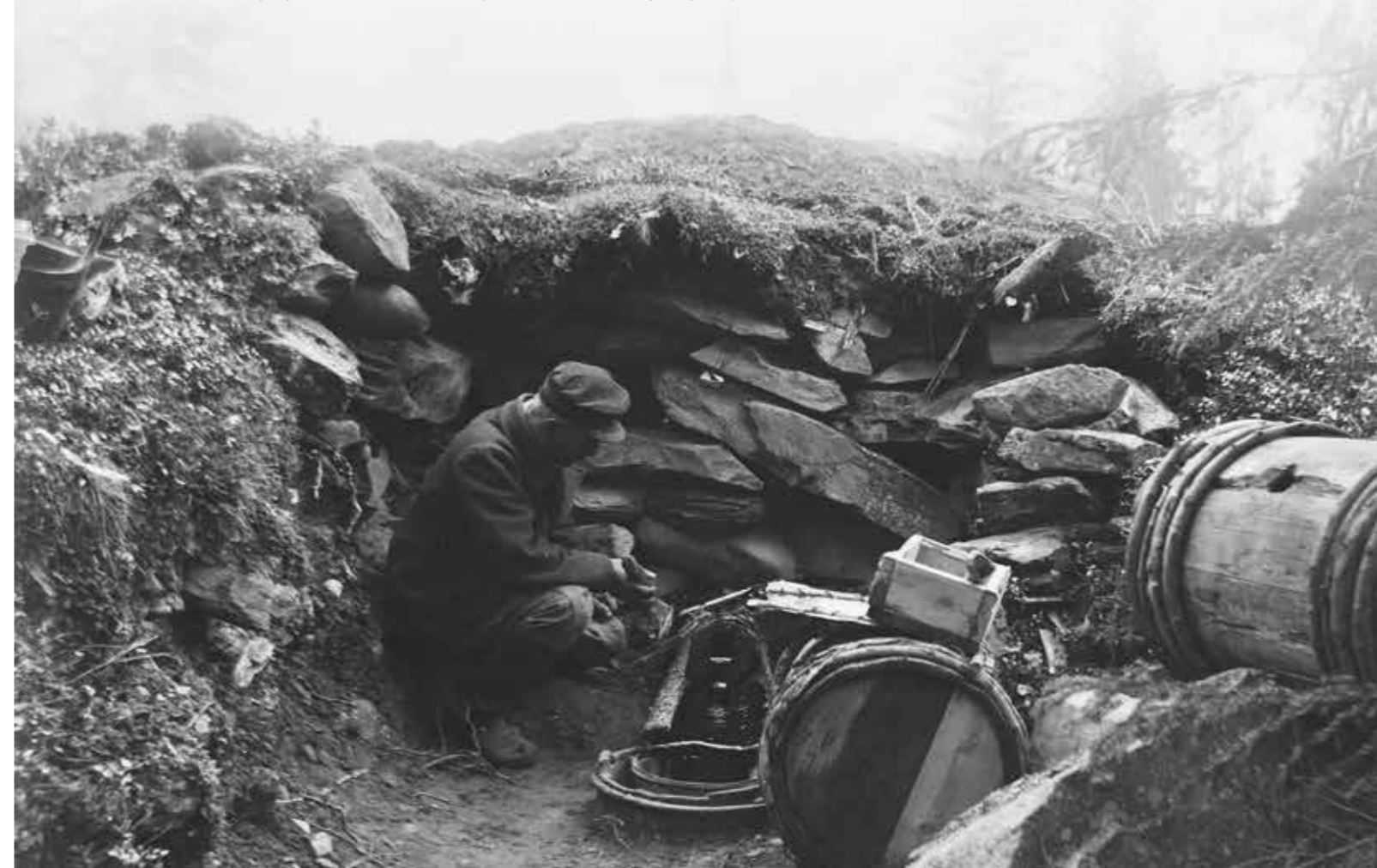
◆ Hot tar flowed down through a pipe into containers. Once cooled, it was transferred into standard 124.8-litre barrels and transported to ports via rivers and lakes. Samuli Paulaharju, the Samuli Paulaharju Collection, the Ethnographic Picture Collection, the Finnish Heritage Agency.
