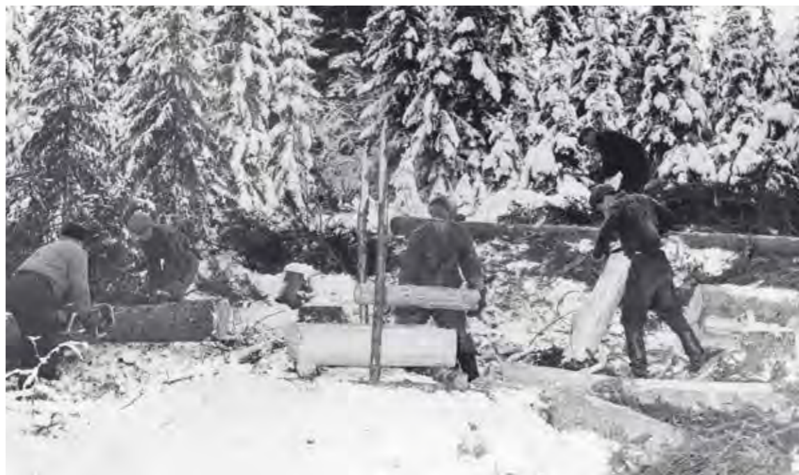
◆ Chainsaws were introduced on logging sites in the 1950s. They were heavy and required two men to operate. Chainsaws were used to fell trees and cut them to length, while branches were lopped off with axes and logs were debarked in the forest using bark spuds and peeling irons. In this image, a five-man crew make spruce pulpwood in a G. A. Serlachius Ltd forest. G. A. Serlachius Ltd, Serlachius Museums.
