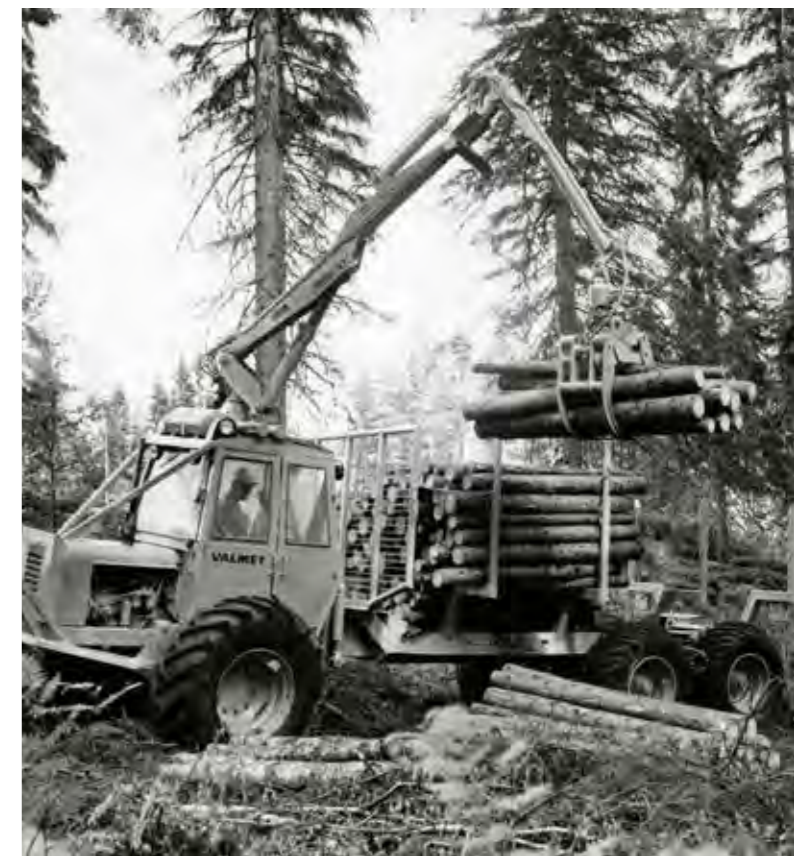
◆ With forwarders, timber could be quickly transported to roadside landings to await onward transport. In this image, a Valmet forwarder loads spruce pulpwood onto a trailer. Valmet Oy, Lusto.
